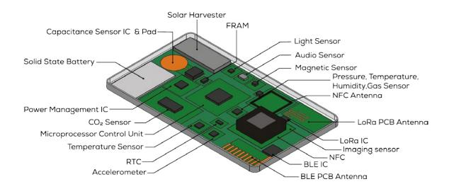
In this phase, AMANDA members are focused on fine-tuning the architecture design of the AMANDA device and defining a high-level overview of the components. The project is focused on functionality design and system miniaturization to increase flexibility, allowing for multiple iterations during the integration process.
