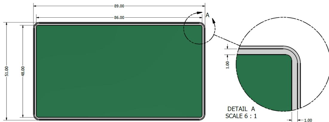
Figure 10 PCB and device enclosure dimensions
