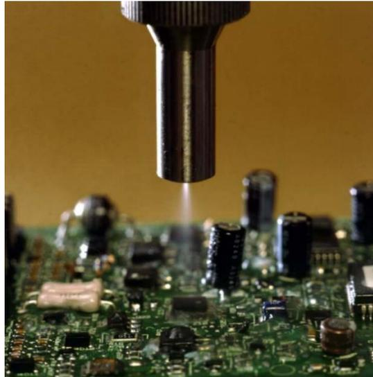
Figure 15 Conformal coating encapsulation method [7]
