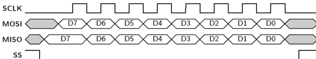
Figure 7 SPI frame
