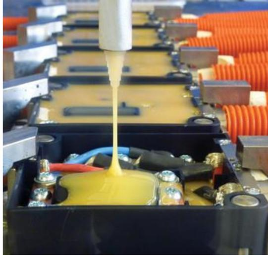
Figure 14 Potting encapsulation method [6]
