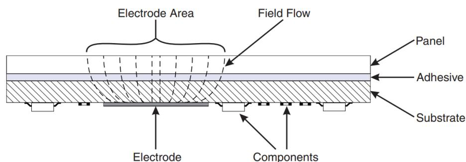
Figure 12 Example „Back-firing“ capacitive sensor layer stackup [5]
